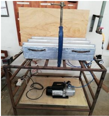
Figure 7. Completely Assembled PV Panel Laminating Machine
